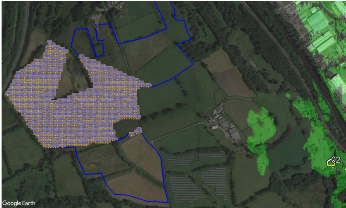
Figure 25 Visible terrain (green areas) from 2m agl at dwelling receptor 02 - Google Earth viewshed image
