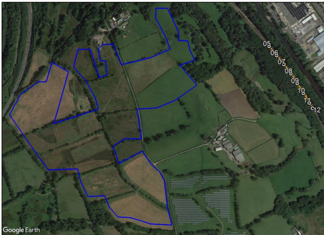
Figure 27 Section of railway towards which solar reflections are geometrically possible (orange) – aerial image
